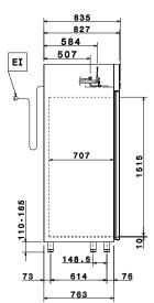
El = Electrical inlet (power) RI = Refrigerant Inlet = Refrigerant Outlet
